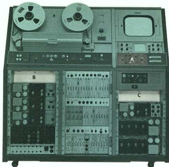
Mark I Editec as installed on the VR-2000B. (A) is Editec Control Panel; (B) is Editec Program Unit; (C) is the Mark III Electronic Editor.
