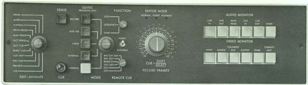
Mark I Editec Controls and VTR Monitor Switching Panel
