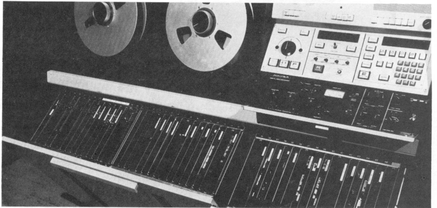
Ampex engineers Maurice Lemoine, left, and Joachim Diermann captured a record SMPTE audience's rapt attention with a remarkable demonstration of digital video. The system was housed in a standard VPR-3 quadruplex VTR cabinet, but the electronics bay (below) in the base contained an impressive array of new PC boards to yield striking digital pictures.
